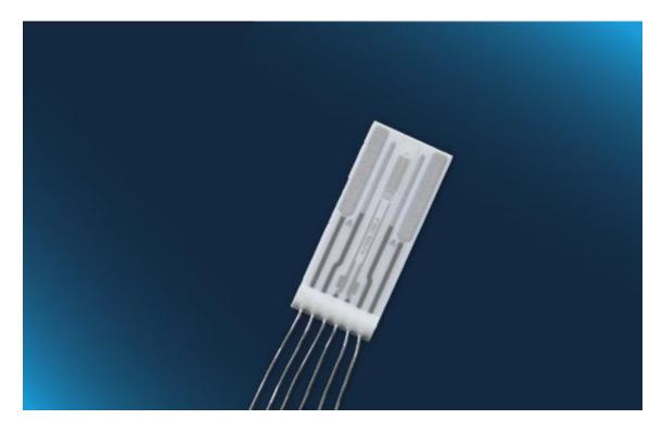
Optimal for applications with a conductivity measuring range from 100  $\mu$ S/cm to 200 mS/cm (typical cell constant of 0.68 cm  $^{-1}$ ) with integrated Pt1000 temperature sensor
