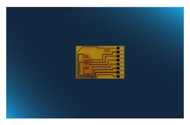
Flow range from 0 to 1.5 m/s (full bridge mode), -20 °C to +80 °C, fast response time
