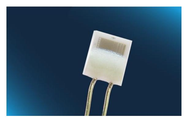
Small thin-film platinum 100 Ohm RTD component, temperature range -200 °C to +600 °C, 1.6 x 1.2 mm, 10 mm wires
