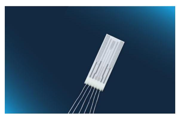
Optimal for applications with a conductivity measuring range from 100  $\mu$ S/cm to 200 mS/cm (typical cell constant of 0.68 cm  $^{-1}$ ) with integrated Pt1000 temperature sensor
