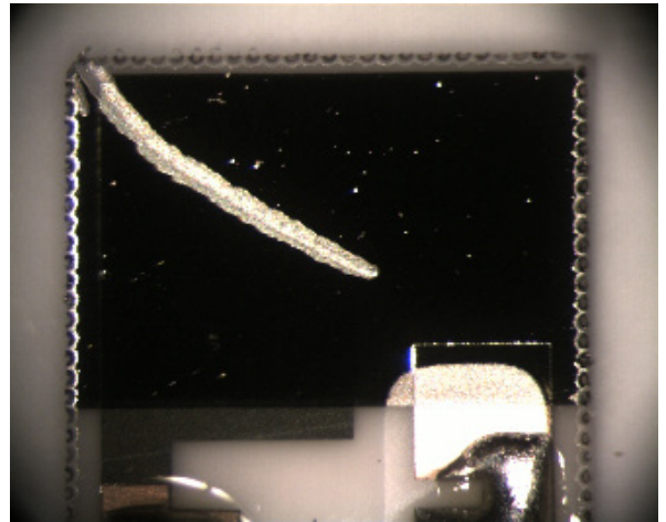
Picture 8: Sensor with a scratch
