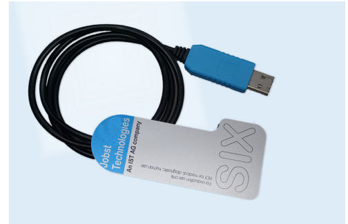
„Six“ with housing and USB connector
