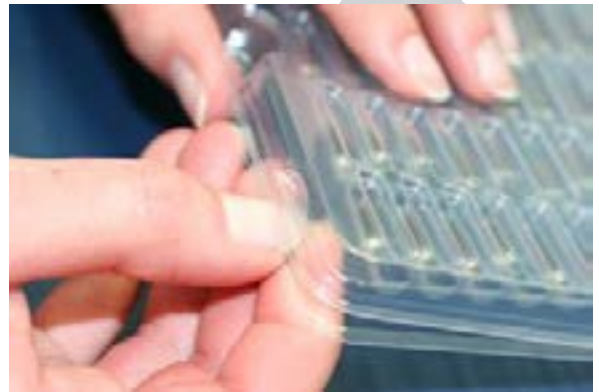
2. Push your thumb beneath cover and press carefully lock system until cover removes smoothly.
