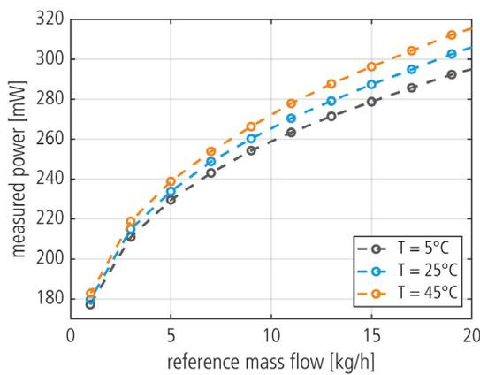
Fig. 5: Heating power as a function of the mass flow for three temperatures
