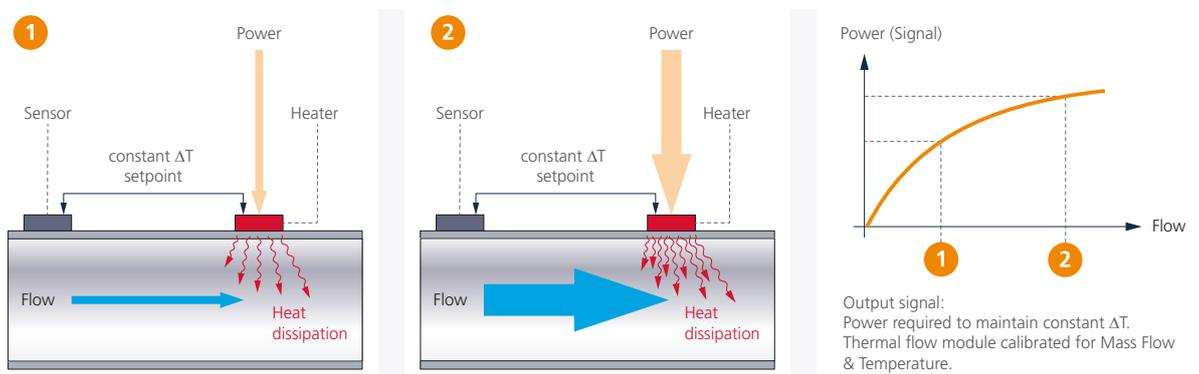
Fig. 1: Anemometric measuring principle
