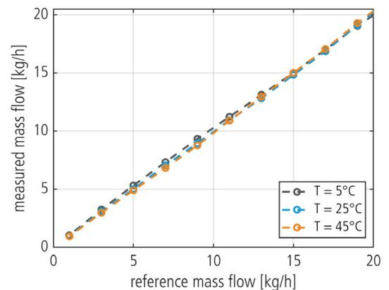
Fig. 6: Linearized and temperature compensated signal of OOL module as a function of the mass flow of reference
