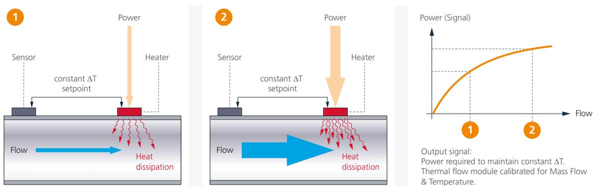
Fig. 1: Anemometric measuring principle
