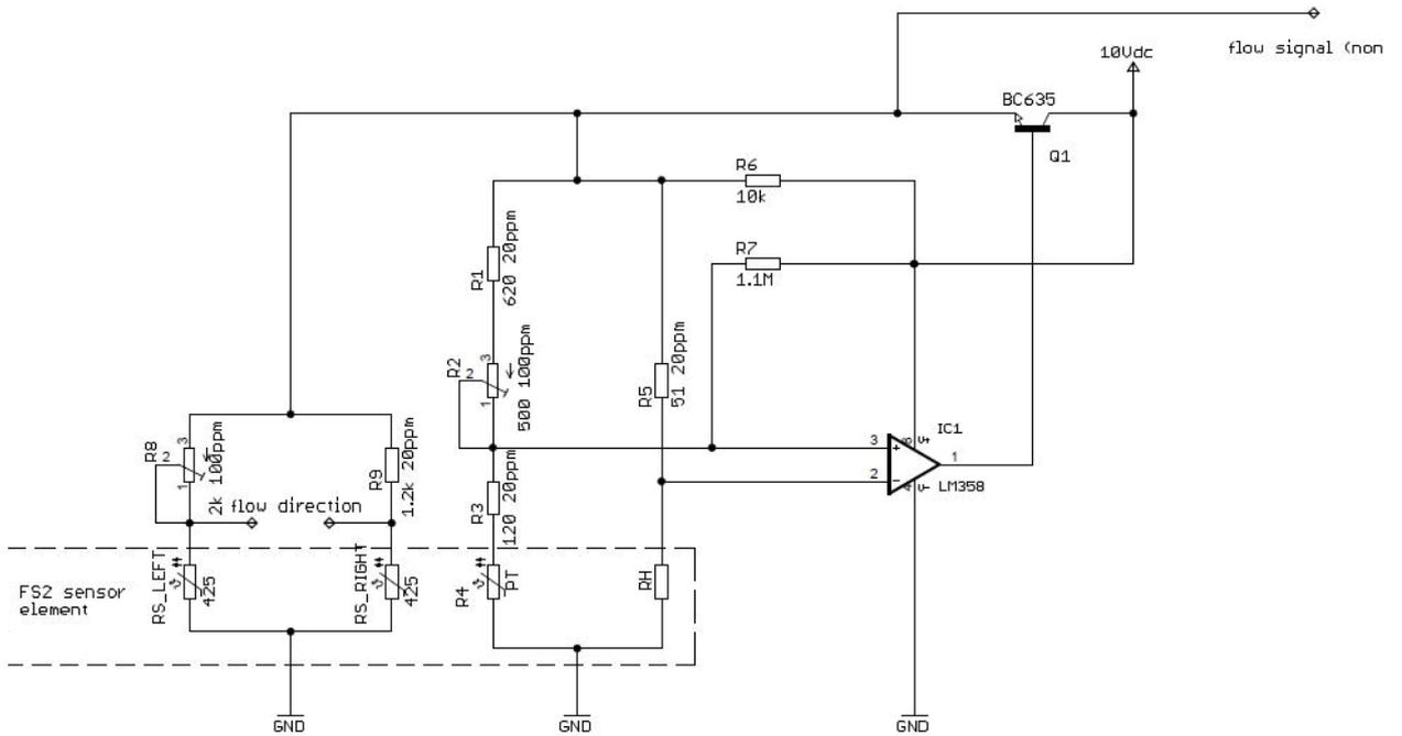
Electronic circuit and curve progression are examples. Each application linked to the accuracy level requires an individual calibration of the system.
