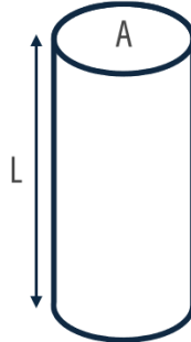
Figure 1-1 Graphical representation of the geometrical factors of a solid conductor
