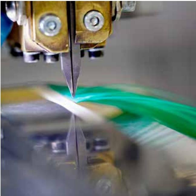
Welding of wires to the sensor
