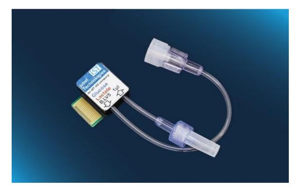
Flow-through biosensor for multiparametric measurement (Glucose and Lactate as standard).
