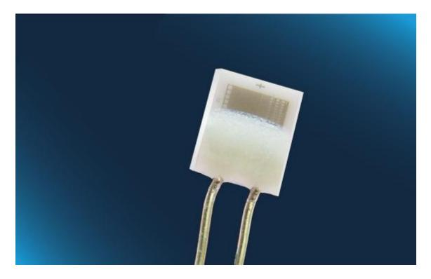
Small thin-film platinum 100 Ohm RTD component, temperature range -200 °C to +600 °C,  $1.6 \times 1.2$  mm, 10 mm wires
