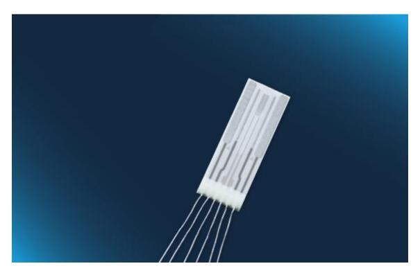
Optimal for applications with a conductivity measuring range from 100  $\mu$ S/cm to 200 mS/cm (typical cell constant of 0.68 cm<sup>-1</sup>) with integrated Pt1000 temperature sensor
