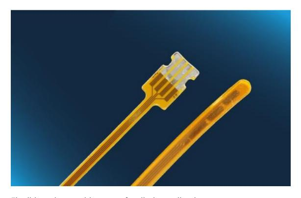
Flexible strip-type biosensor for dip-in applications
