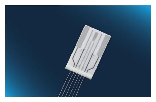
Optimal for applications with a conductivity measuring range from 0.2 mS/cm to 200 mS/cm (typical cell constant of 0.44 cm  $^{-1}$ ) with integrated Pt1000 temperature sensor
