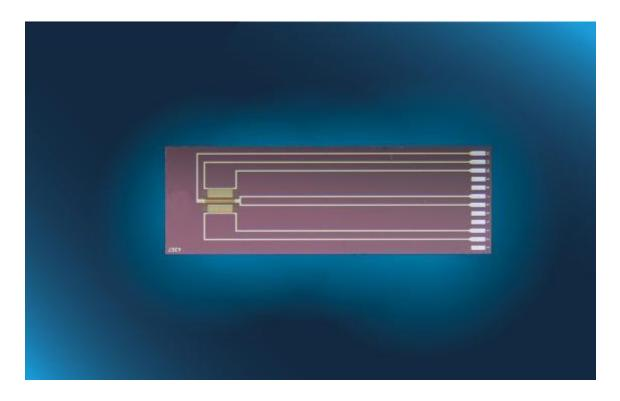
Optimal for fast measuring of gas flow and direction
