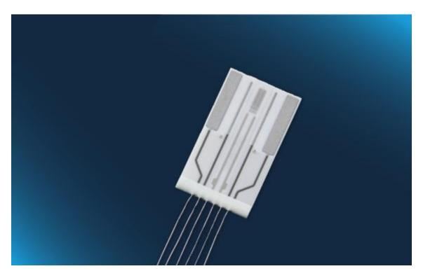
Optimal for applications with a conductivity measuring range from 0.2 mS/cm to 200 mS/cm (typical cell constant of 0.44 cm<sup>-1</sup>) with integrated Pt1000 temperature sensor
