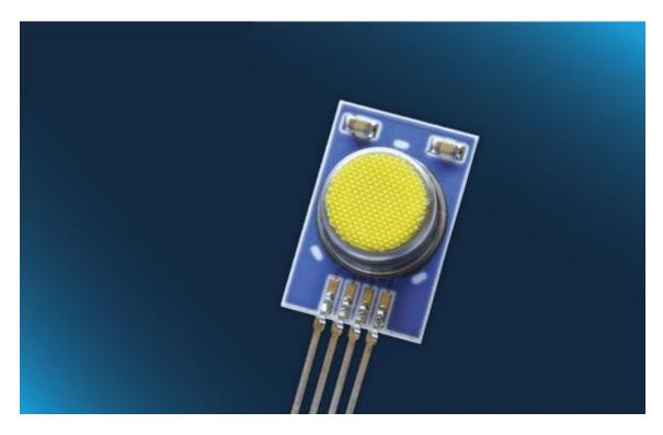
Digital RH/T module with compact dust filter, suitable for HVAC
