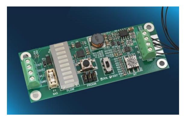
Flow Demo Board with FS7 Sensor: evaluation electronics for anemometric (thermal) flow sensors
