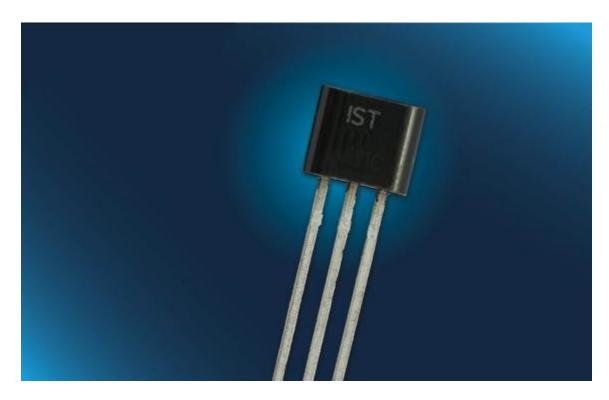
Analog Temperature Sensor Tsic -50°C to 150°C
