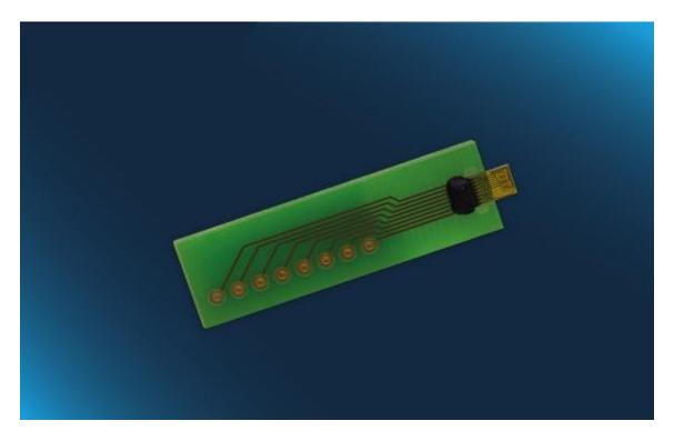
Gas flow sensor with flow range from 0 to 1.5 m/s (full bridge mode), temperature range from -20  $^{\circ}$ C to +80  $^{\circ}$ C, fast response time, mounted on a PCB for easy integration
