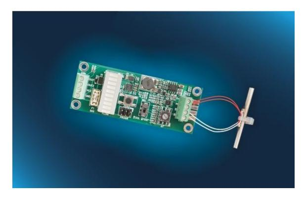
Flow Evaluation Board FS/OOL + OOL liquid sensor. Evaluation electronics for anemometric (termal) flow sensors
