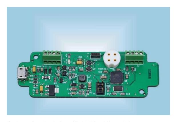
Testing and evaluation board for HYT humidity modules
