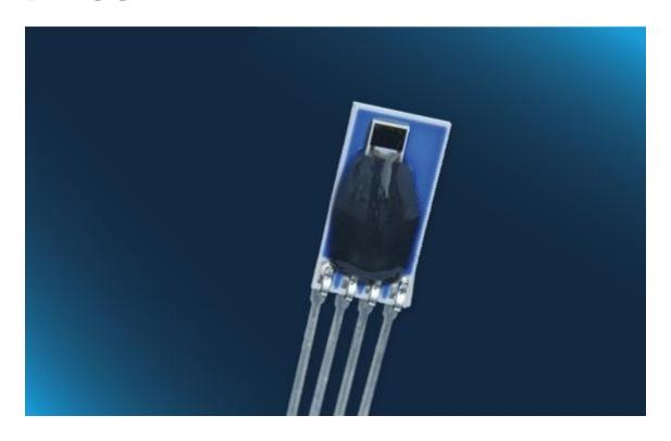
Digital RH/T module, for up to 125°C and 100% RH, withstands condensation
