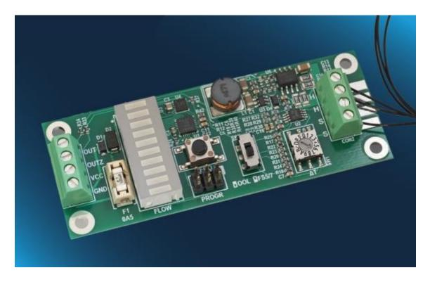
Flow Demo Board with FS7 Sensor: evaluation electronics for anemometric (thermal) flow sensors
