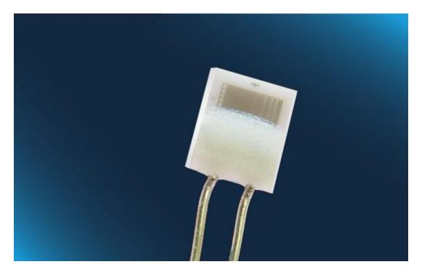
Small thin-film platinum 100 Ohm RTD component with high accuracy, temperature range -200  $^{\circ}$ C to +600  $^{\circ}$ C, 1.6 x 1.2 mm, 10 mm wires
