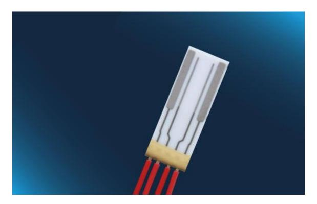
Commodity conductivity sensor with four-electrode measurement. Measuring range from 1000  $\mu$ S/cm to 100.000 mS/cm (typical cell constant of 0.66 cm<sup>-1</sup>)
