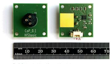
Fig. 2: Driving circuit board for a quick evalution of HISbasic series IR emitters.
