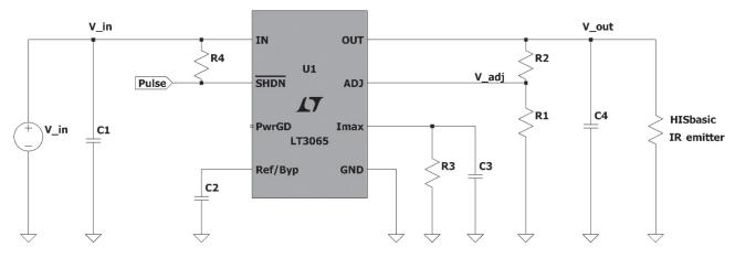
Fig. 1: Application circuit to drive HISbasic series IR emitters with the LDO regulator LT3065
