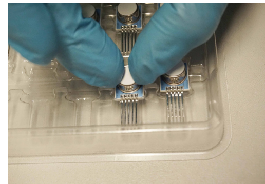
4. Use plastic tweezers only to handle the module
