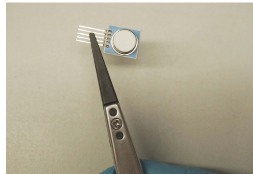
4. Use plastic tweezers only to handle the module
