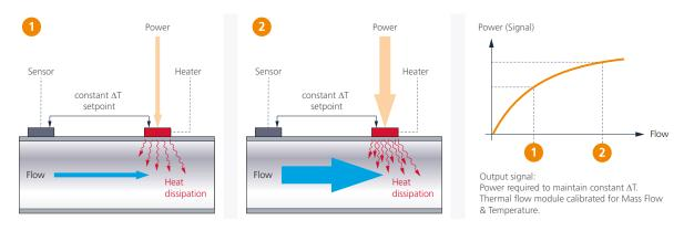
Fig. 1: Anemometric measuring principle
