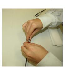
Carefully remove the plastic spiral around the wires
