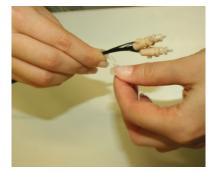
Carefully remove the plastic spiral around the wires
