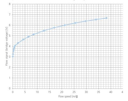
The output signal is adjusted to 3.0 V at zero flow and corresponds to a temperature difference (heater temperature minus ambient) of approximately 30K. With the temperature difference an optimal overhead of the heating element is generated and hence a perfect performance exists. According to King's Law, which is declared in section 1.12, the sensor performance has the highest sensitivity at lower flow speeds.
